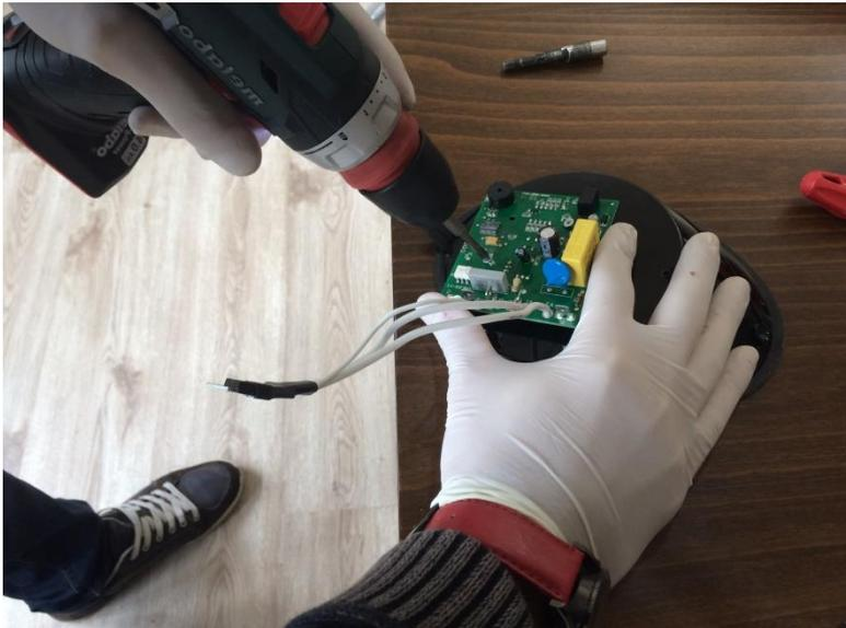
Step 5: Remove the three screws on the Control board
